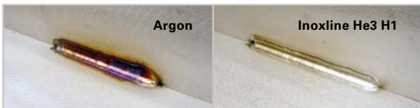
Less oxidation tint with greater sheet thicknesses
